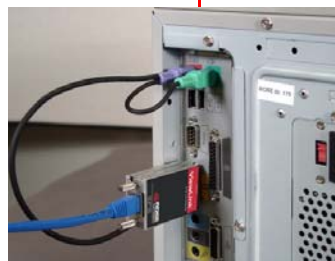
Connect the transmitter directly to a PC's Video, keyboard, and mouse ports
